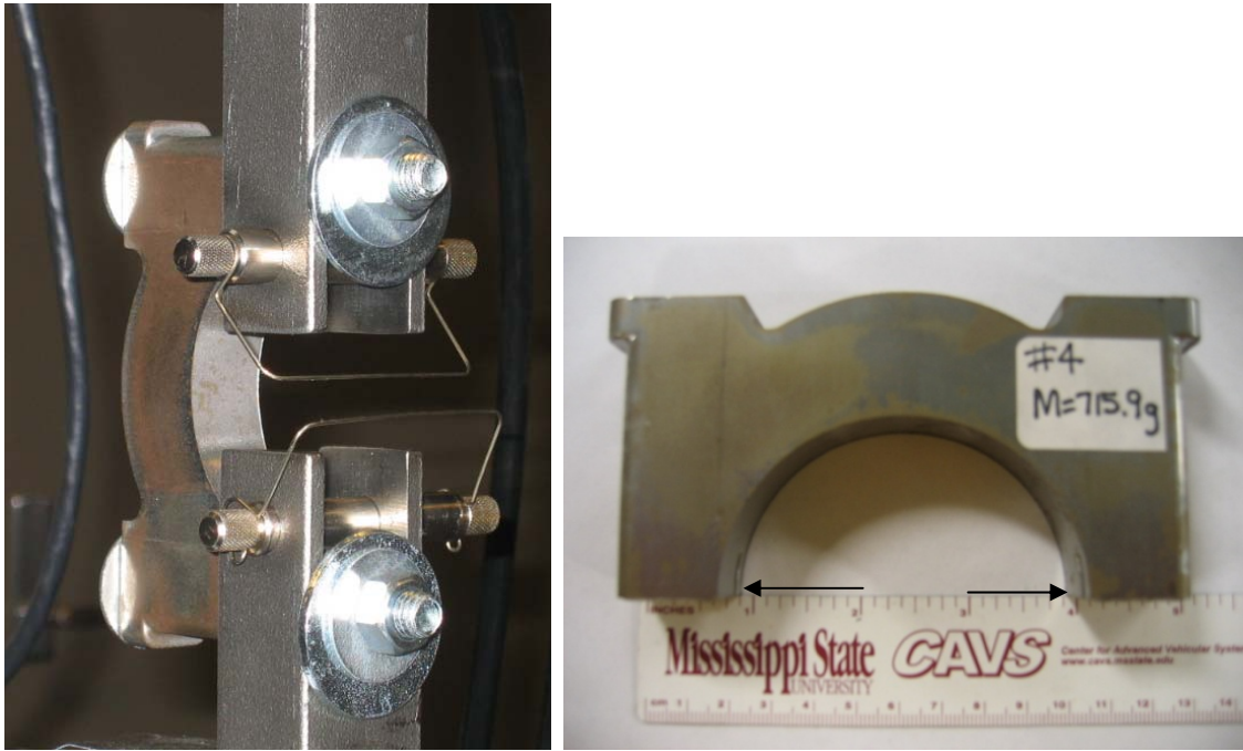
Figure 4.19 Test fixture and loading application of the MBC.
